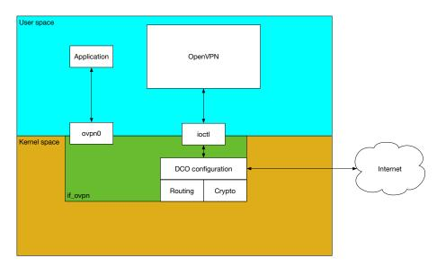
This moves the data channel down into the kernel, removing the need for copies to and from user space.
