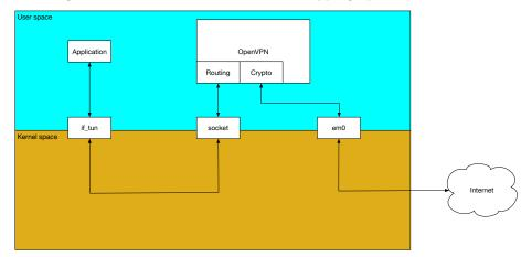
The main issue with OpenVPN's performance is its user space nature. Incoming traffic is naturally received by a NIC, which would typically DMA the packet into kernel memory. It is then processed further by the network stack until that works out what socket the packet belongs to, and passes it to user space. This socket may be UDP or TCP.
